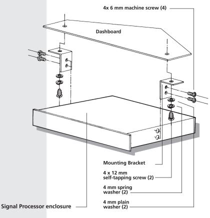
This Half-DIN size unit can also be installed in the dash adjacent to the head unit, provided that there is a slot available.
